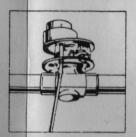
2. Loosen the 2 small set screws (on earlier models — Allen screws) protruding through bottom mounting plate. Turn only the operator counter-clockwise until screws line up with enlarged holes in end of slot. Do not turn mounting plate.
