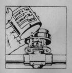
1. Remove cover by loosening 2 securing screws located on sides.
